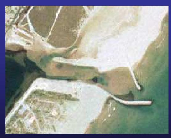
Construction of two breakwaters situated on either side of the mouth of a river flowing into the sea.
