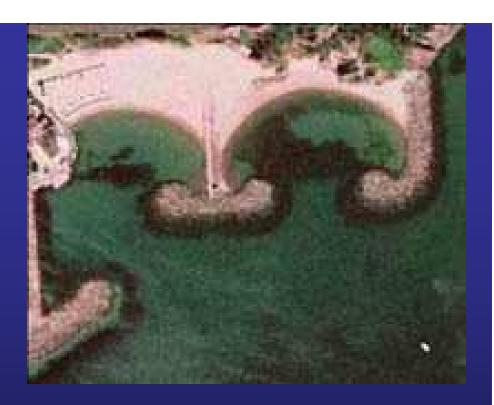
Breakwater protected beach: development consisting of two rocks dump breakwaters, curving inwards towards each other at the seaward end and delimiting an area reclaimed land and a sheltered stretch of water for bathing
