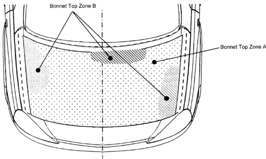
3.3.2 Marking of the “Bonnet Top” impact area as well as “Bonnet Top Zone A” and “Bonnet Top Zone B” will be based on a drawing supplied by the manufacturer, when viewed from a horizontal plane above the vehicle that is parallel to the vehicle horizontal zero plane. A sufficient number of x and y co-ordinates shall be supplied by the manufacturer to mark up the areas on the actual vehicle while considering the vehicle outer contour in the z direction.
