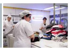
Laundry ID not only eliminates sorting errors, but also standardises the labelling process by attaching a water and heat resistant label containing a reusable radio-frequency identification chip to each garment. It identifies the garment while the worker is folding it, showing who the owner is on a screen. A light in the shelves is illuminated to indicate where the garment should be left for distribution.
